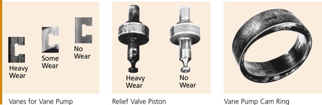
Figure 1. Typical Examples of Wear Due to Contamination
